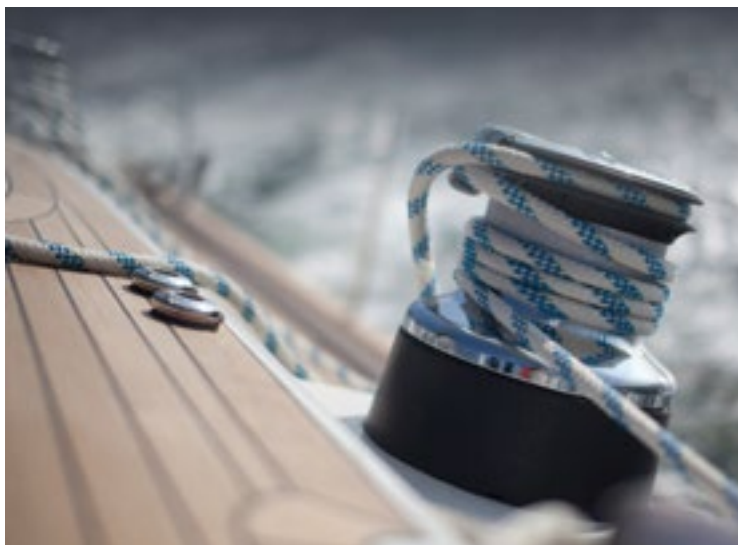
Electric Evo 80 installed on Hallberg Rassy
